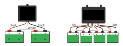
Failure to use an external battery balancer will result in damage, severe degradation and voiding of warranty.
